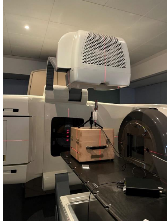
Figure 23. CBCT aligned with the detector equipped with the Tungsten collimator at 40 cm.
