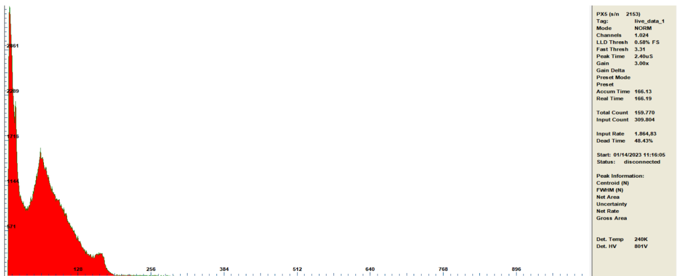
Figure 58. Raw spectrum 80 kV, linear scale, gain 3x.
