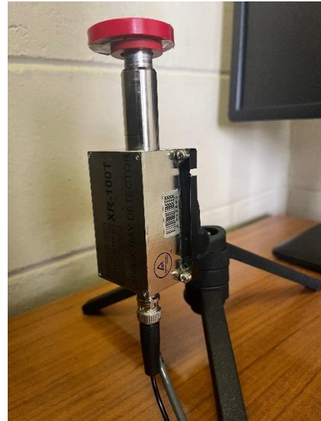
Figure 21. XR-100T-CdTe Gamma Ray and X-Ray Detector with ^{241}\text{Am} & ^{152}\text{Eu} Radionuclides on top.
