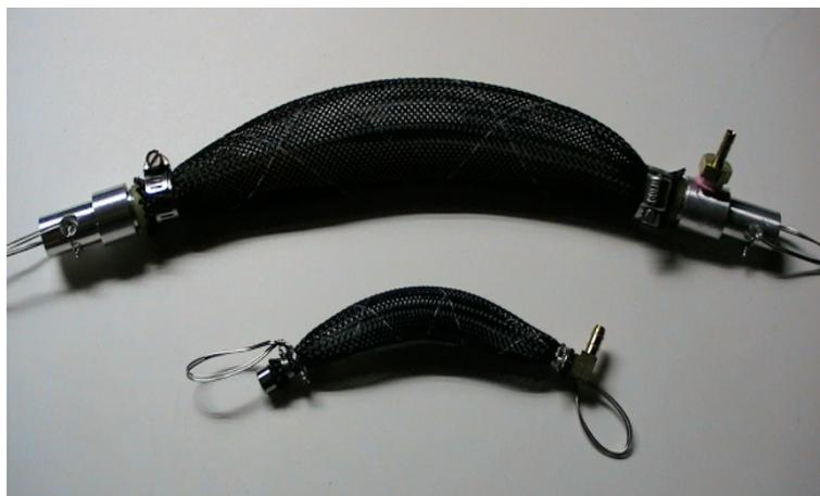
Figure 2.6: Example of Pneumatic artificial muscle.
