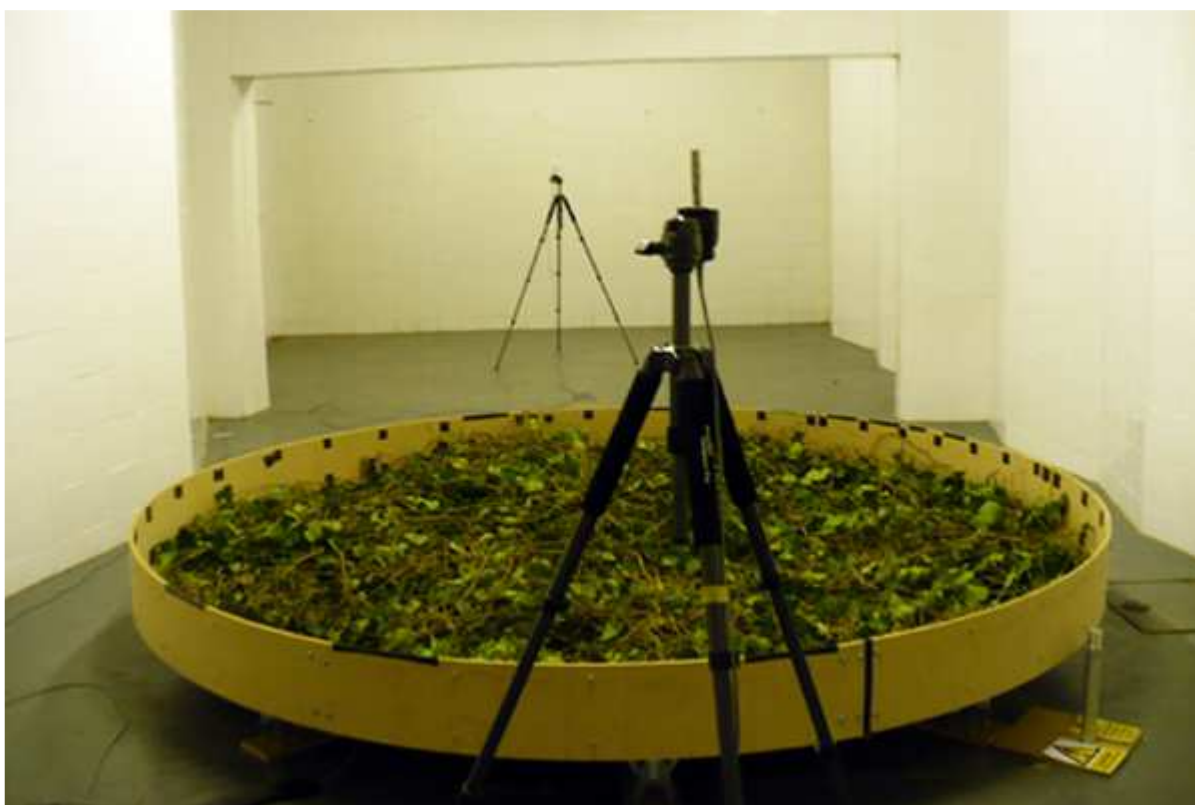
Figure 3. The turntable with Ivy into the Reverberation Chamber of the University of Sheffield
