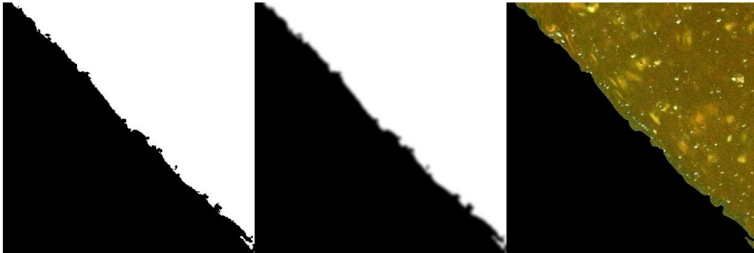
Figure 74 Three main process to obtain the body domain (optimised for the lower surface) as shown in Fig. 76. On the left: binarization of the photo obtained by the subtraction of the blue channel from the red channel. In the middle: Gaussian filter applied to the previous photo. On the right: Binarization of the photo in the middle and multiplication by the original photo.
