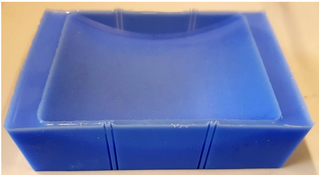
Figure 57 Concave mould base to realise a hard candy block with a convex face. In cross-sectional view the surface is an arc of circumference of diameter 170 mm. The two lines of points made of the extrema of the arc of circumference are 125 mm apart.
