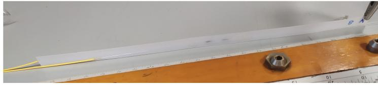
**Figure 6.9:** Picture of the sensor built to study the case of a two-dimensional strain.
