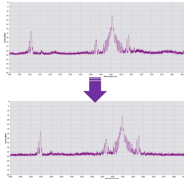
Figure 8.3: Effect of traction on one of the sensor gratings.
