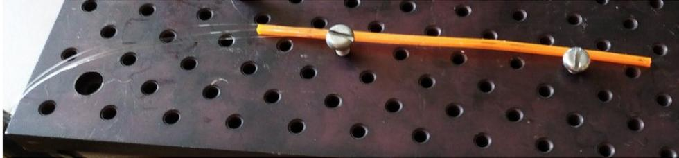
**Figure 8.6:** The sensor obtained pasting the gratings to the substrate along their entire length.
