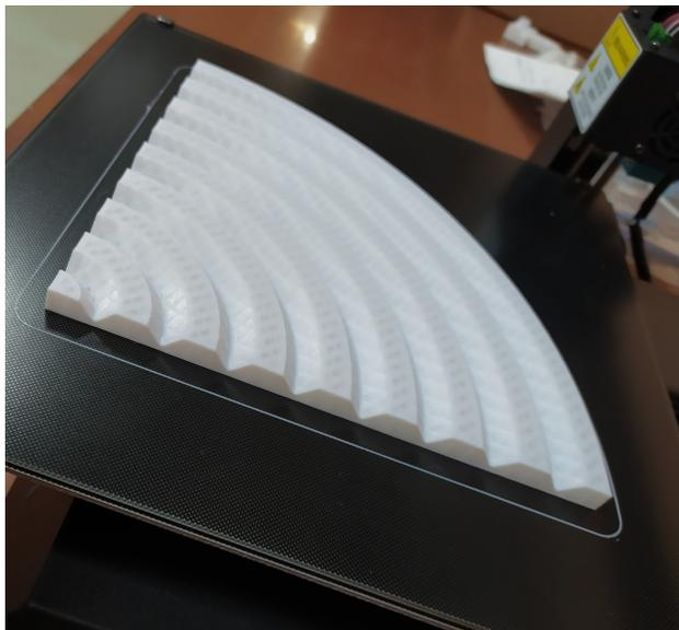
**Figure 6.6:** The realised calibration board in white PLA.
