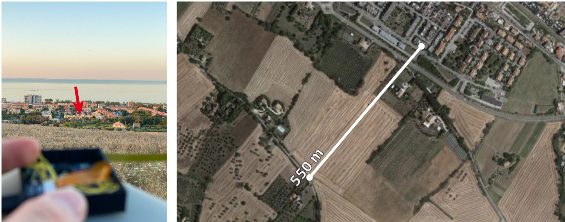
Figure 4.16: Communication Test over 550 m in line-of-sight.
