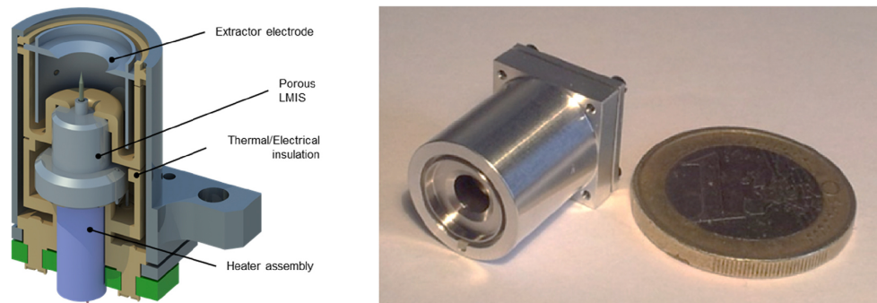
Figure 3.21: NanoFEEP Thruster head: a detailed schematic (left) and a photo of a manufactured prototype [73].
