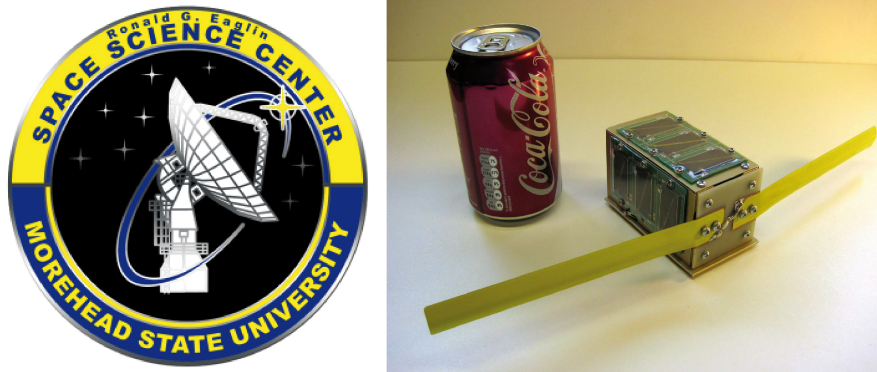
Figure 1.10: Eagle-2 also known as $50SAT, 1.5P PocketQube from Morehead State University (USA) [15][16]. It can be noticed the Backplate used for deployment.
