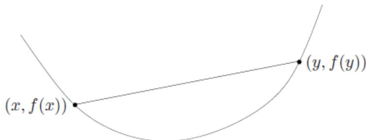
**Figure 2.7:** Graph of a convex function  $f(\cdot)$ , where the line segment between two generic points  $(x, f(x))$   $(y, f(y))$  lies above the function itself [6].
