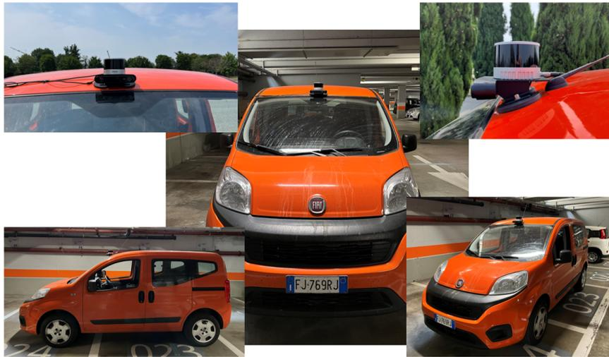
Figure 3.14: LiDAR and camera mounting position
