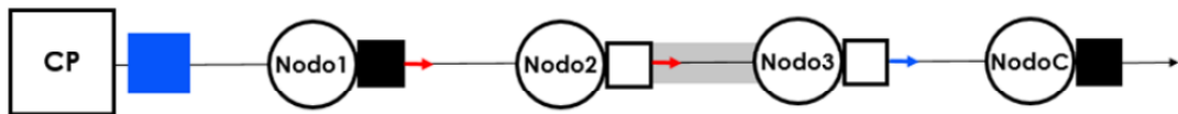
Figure 2.36: The end-of-line substation receives the message and closes its switch to allow power coming in through a neighbouring line to power back the users affected by the fault. [16]
