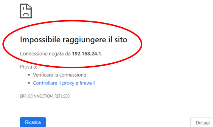
(b) Firewall is on, a connection can not be established through the WAN interface to the virtual router.
