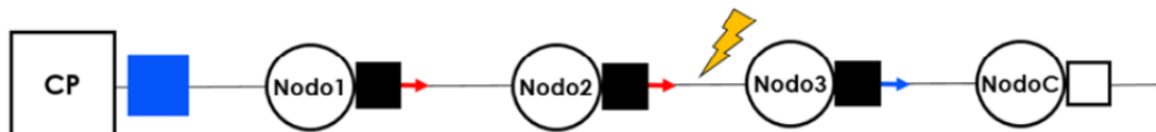
Figure 2.28: A fault occurs between "nodo 2" and "nodo 3", the primary substation, "nodo 1" and "nodo 2" are all able to sense the fault.[16]
