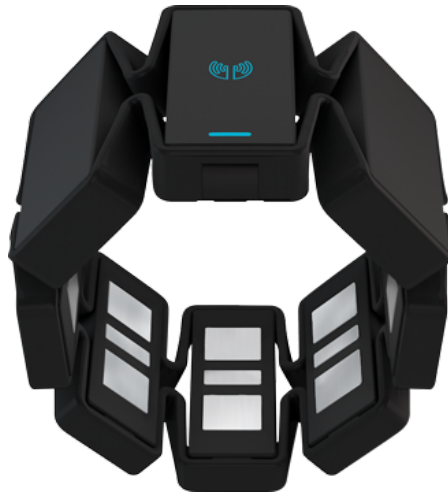
Figure 3.16: Myo Armband Sensor from North Inc.
