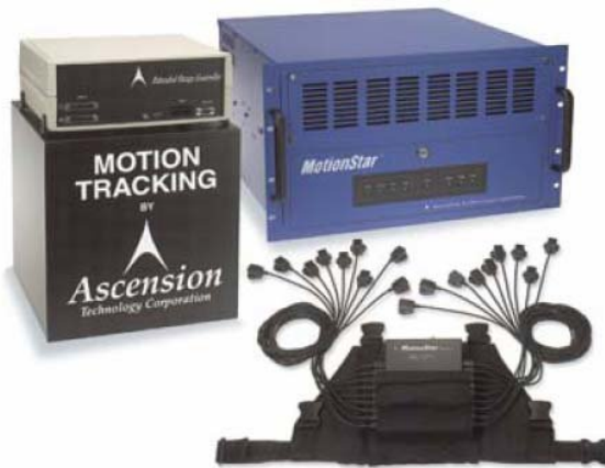
Figure 3.2: MotionStar DC magnetic tracker by Ascension Technology Corporation
