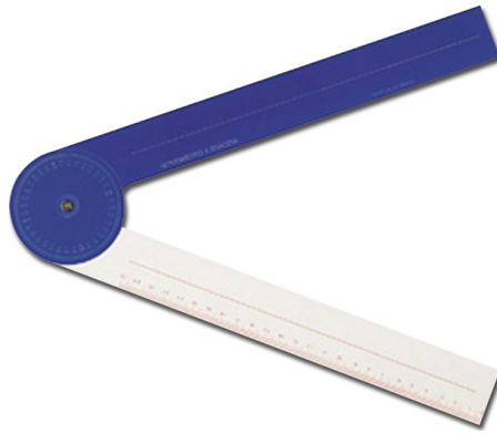
Figure 3.7: universal goniometer for anthropometric measurements
