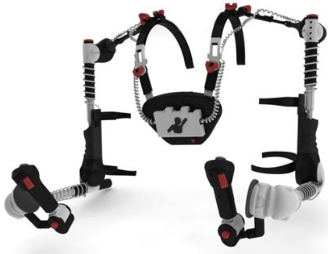
Figure 3.3: Gypsy 7 Torso Motion Capture System
