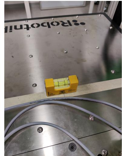
(c) Level placed on top of the chassis to ensure that it is parallel to the ground
