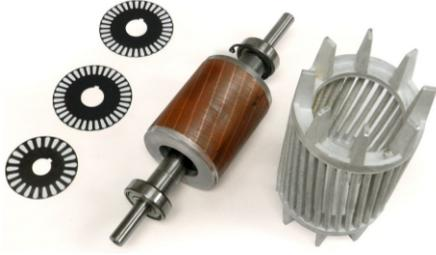
**Figure 1.10:** Squirrel cage rotor for an IM
