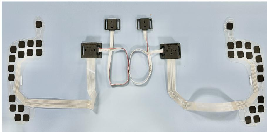
**Figure 4.5:** INDIP System with PI, IMUs and DS.
