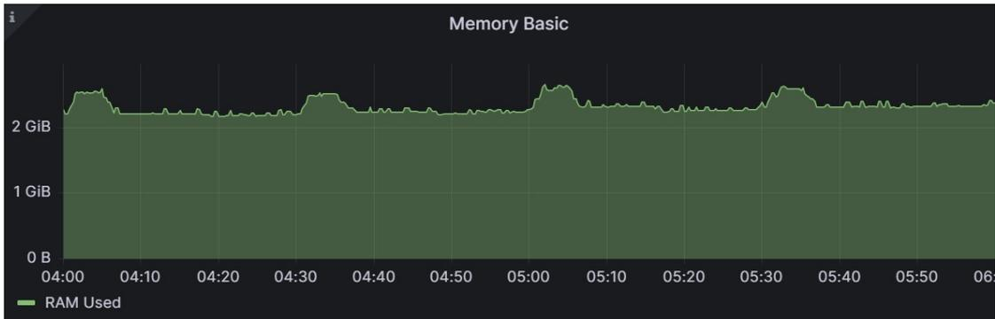
Figure 8.52: Average Edge RAM Utilization for 16 Sensors
