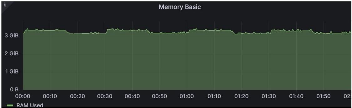
Figure 8.43: Average Centralized RAM Utilization for 4 Sensors
