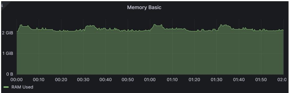
**Figure 8.50:** Average Edge RAM Utilization for 4 Sensors
