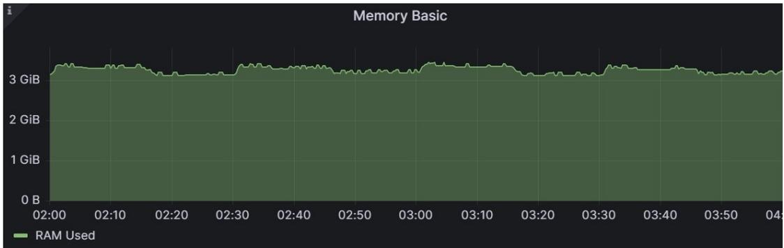
Figure 8.44: Average Centralized RAM Utilization for 8 Sensors
