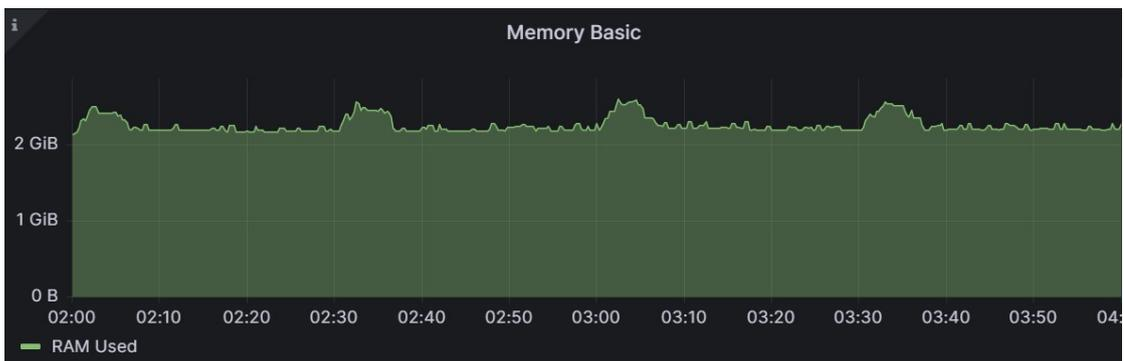
**Figure 8.51:** Average Edge RAM Utilization for 8 Sensors
