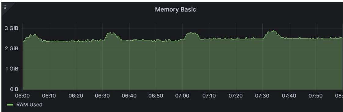
Figure 8.53: Average Edge RAM Utilization for 32 Sensors
