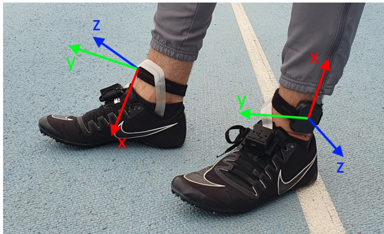
Figure 5.6: Axes orientation of the IMUs
