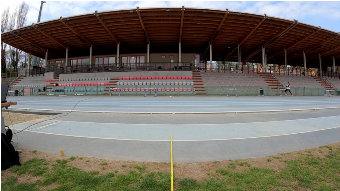
Figure 5.12: Typical look of a wide angle lens, straight lines are bent
