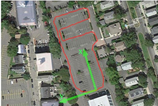
Fig. 2: The robot's path as a mean of the two raw GPS paths is shown in red. Its world coordinate frame is shown in green.
