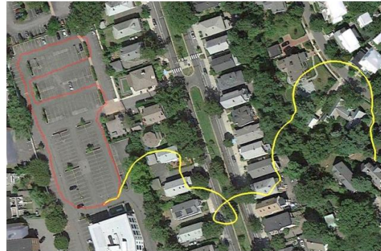
Fig. 3: Output of ekf_localization_node (yellow) when fusing only raw odometry data.
