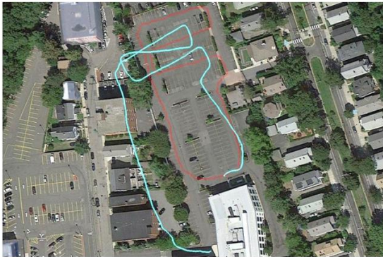
Fig. 4: Output of ekf_localization_node (cyan) when fusing data from odometry and a single IMU.
