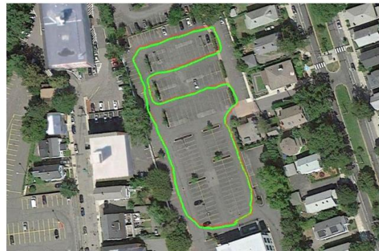
Fig. 7: Output of ekf_localization_node (green) when fusing data from odometry, two IMUs, and two GPS units.
