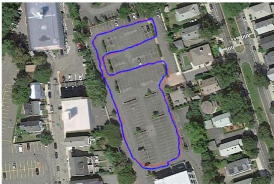
Fig. 6: Output of ekf_localization_node (blue) when fusing data from odometry, two IMUs, and one GPS.
