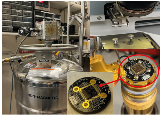
Figure 4.7: On the left, the dipstick probe inserted into the liquid helium dewar. The top right image shows the tip used to wirebond the chip. The bottom right shows the PCB mounted on the probe. Our NbN samples were placed in the middle of a PCB with 28 contact pads for the connections and 0 \Omega soldered resistors.
