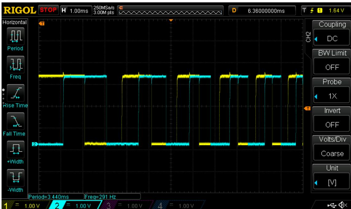
Figure 2.6: Output signal of the encoder (Turning sense 1).
