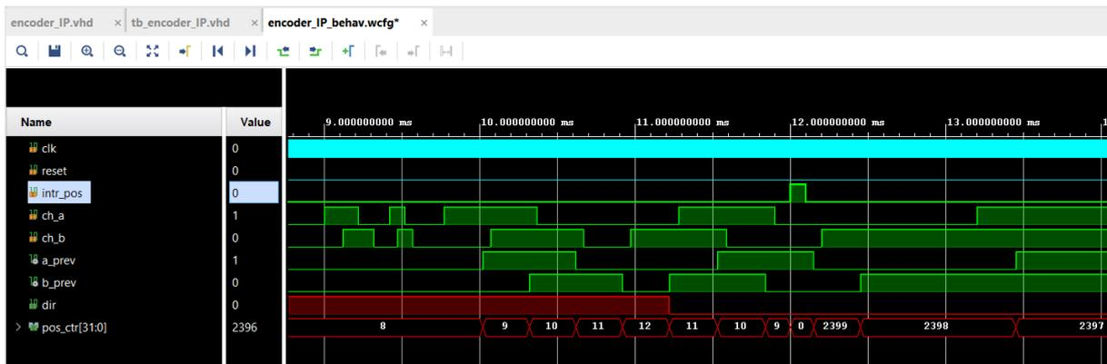
Figure 6.4: Simulation of the Rotary Encoder IP
