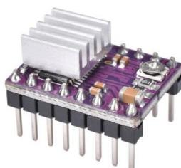
Figure 2.14: The heat sink attached to the motor driver.
