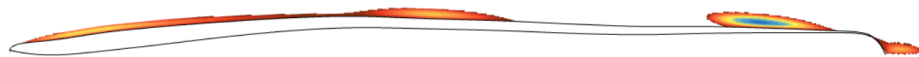
Figure 75: Laminar separation bubbles formed at Re = 10000 and M = 0.5 over the upper surface of ld34-14-7U
