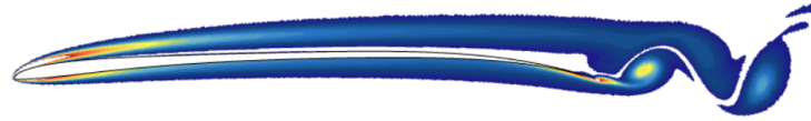
(a) Instantaneous vorticity field of the initial airfoil at Re = 8000 , M = 0.5 and \alpha = 5^\circ
