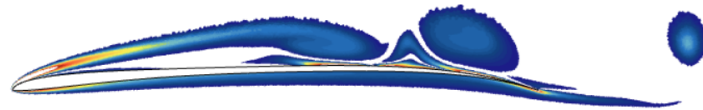
(b) Instantaneous vorticity field of the initial airfoil at Re = 8000 , M = 0.5 and \alpha = 6^\circ
