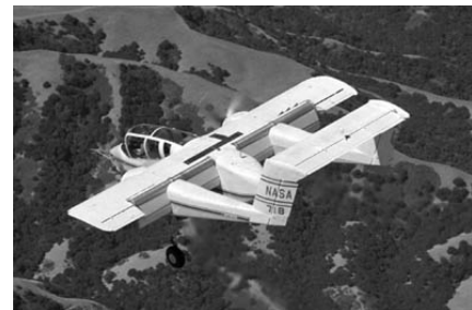
Figure 1.6: NASA YOV-10A prototype with an integrated rotating cylinder flap
