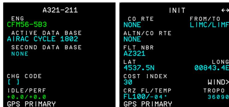
**Figure 5.3:** MCDU pages - DATA A/C STATUS (left) and INIT-A (right)
