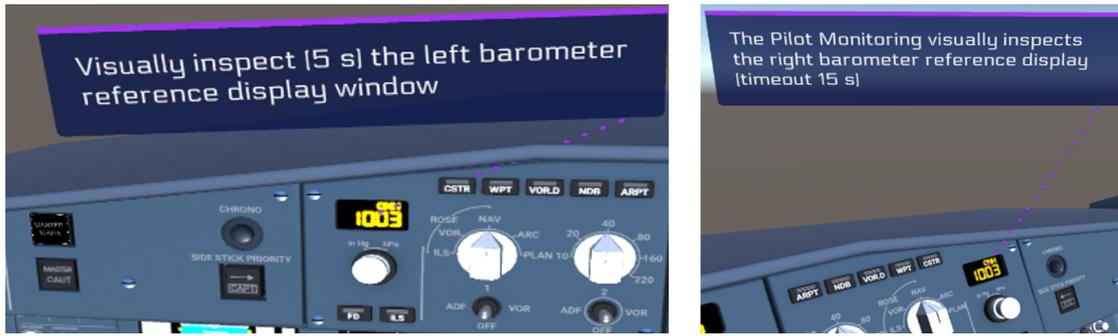
Figure 5.14: Cockpit Preparation: node 17.4 (left) and node 18.4 (right)
