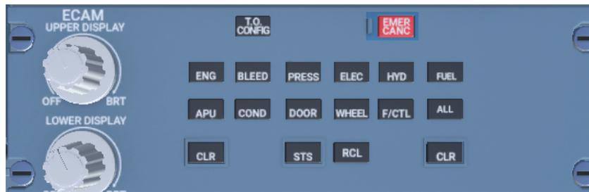
Figure 4.3: ECAM control panel
