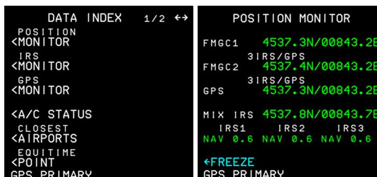
**Figure 5.13: Cockpit Preparation:** MCDU DATA page (left) and DATA - POSITION MONITOR page (right)
