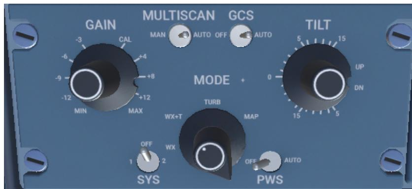
**Figure 4.5:** Weather Radar panel
