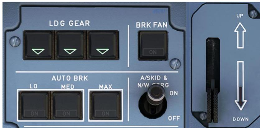
**Figure 4.12:** Autobrake and Gear indications panel
