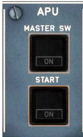
Figure 4.26: APU control panel
