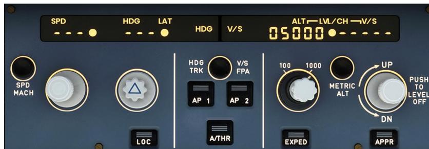
Figure 4.16: Flight Control Unit
