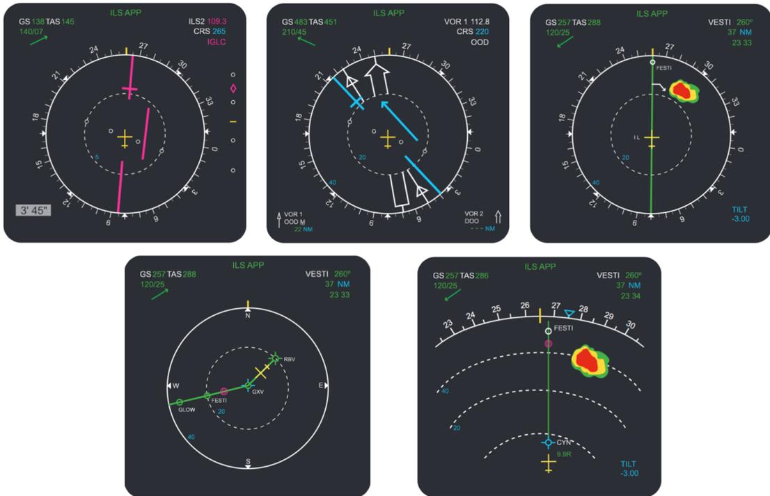
**Figure 4.13:** Navigation Display modes: ROSE ILS, VOR, NAV and ARC and PLAN (left to right, up to down)
