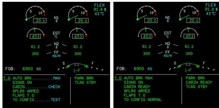
**Figure 5.34: Taxi:** Upper ECAM at the start (left) and at the end (right) of the procedure
