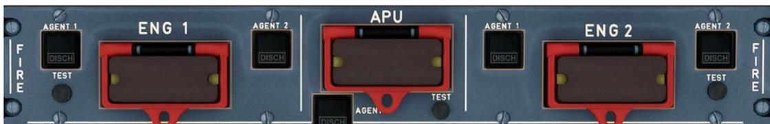
**Figure 4.21:** Fire Control panel
