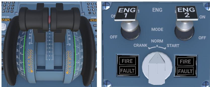
**Figure 4.8:** Thrust levers and Pitch Trim wheel (left) and Engine panel (right)
