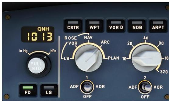
**Figure 4.14:** EFIS control panel
