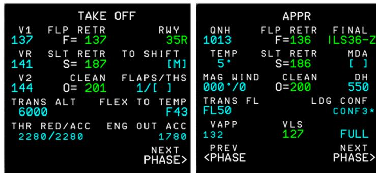
Figure 5.5: MCDU pages - PERF TAKE OFF (left) and PERF APPROACH (right)
