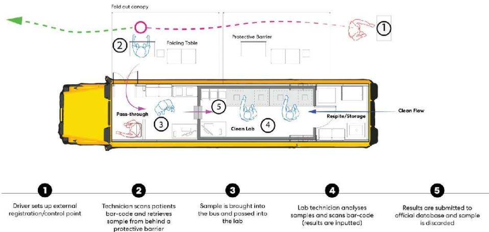
A plan of the Mobile testing center bus
