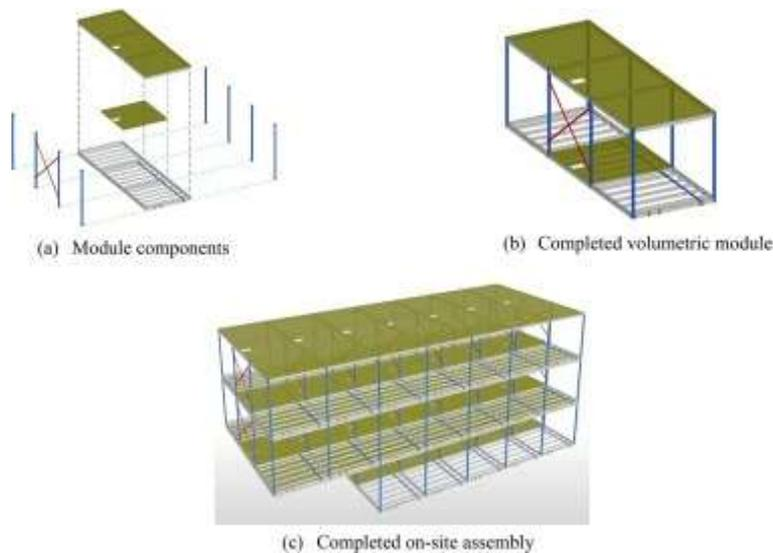
Fig. 1. Modular construction: Module assembly to completed modular building
