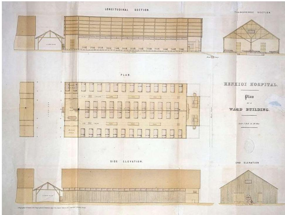
A plan of Renkioi Hospital, a prefabricated hospital from 1855, used during Crimean War.
