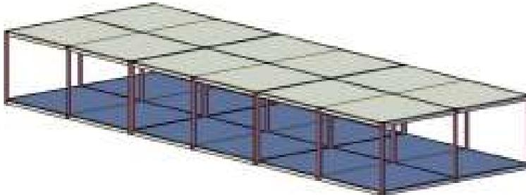
*Fig. 3. Corner post modules arranged horizontally to form wider open space*
