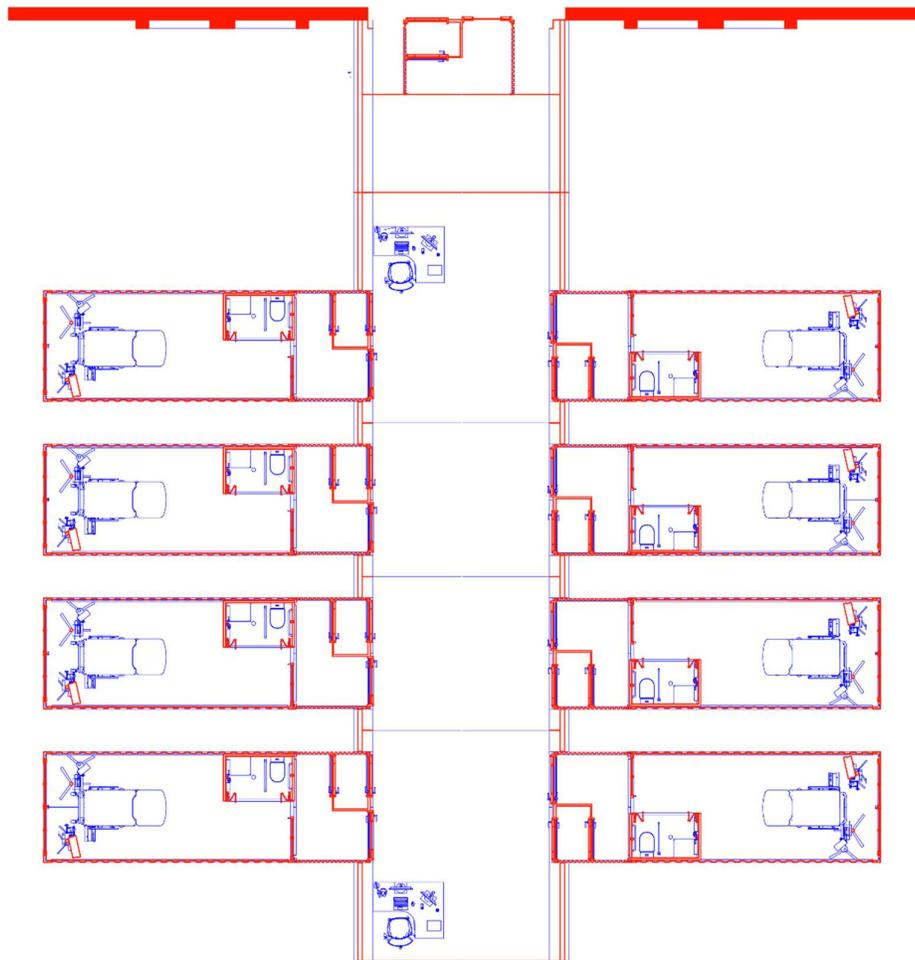
*Drawn: Plan of the modular hospital extension with Filter Space between the inflatable structure and the rooms.*
