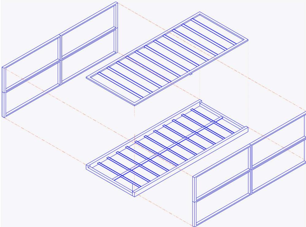
*Drawn: Structural components of a module.*
