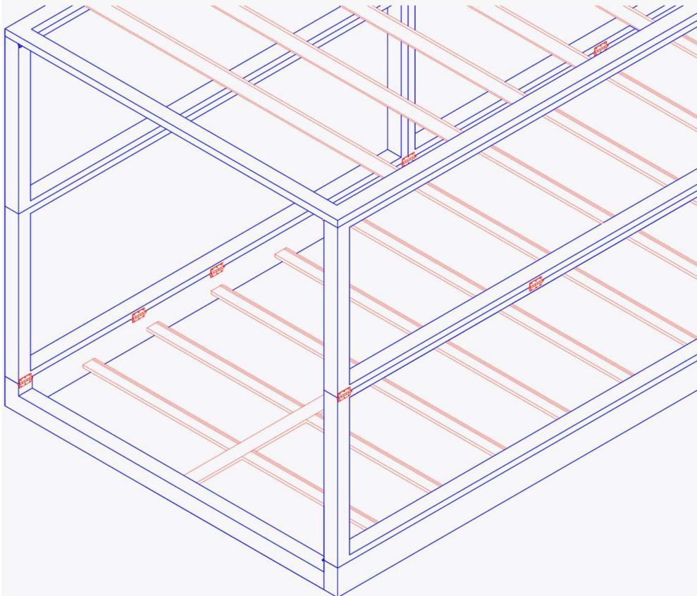
*Drawn: A visual representation highlighting the structure and the hinges used to open the structure.*
