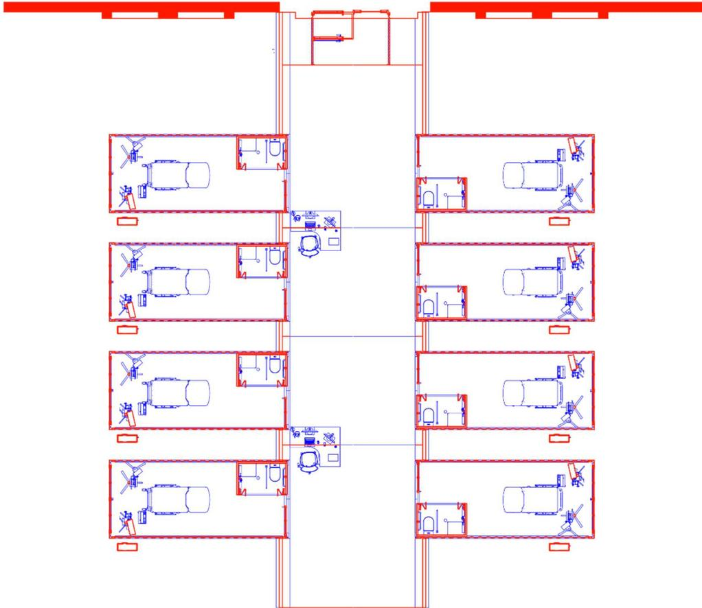
*Drawn: Plan of the modular hospital extension without Filter Space between the inflatable structure and the rooms.*
