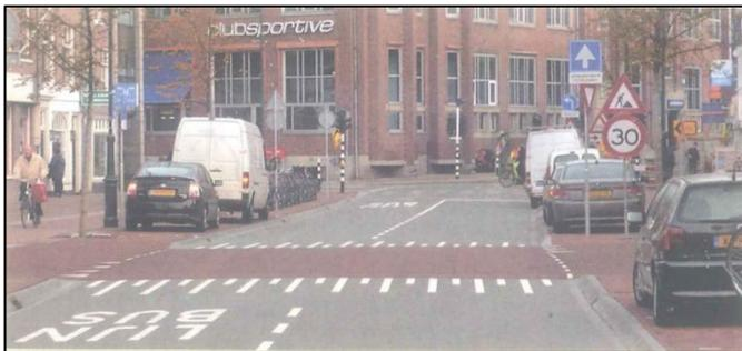
Figure 5-15 Road safety measures: Raising the pavement in the Netherlands
