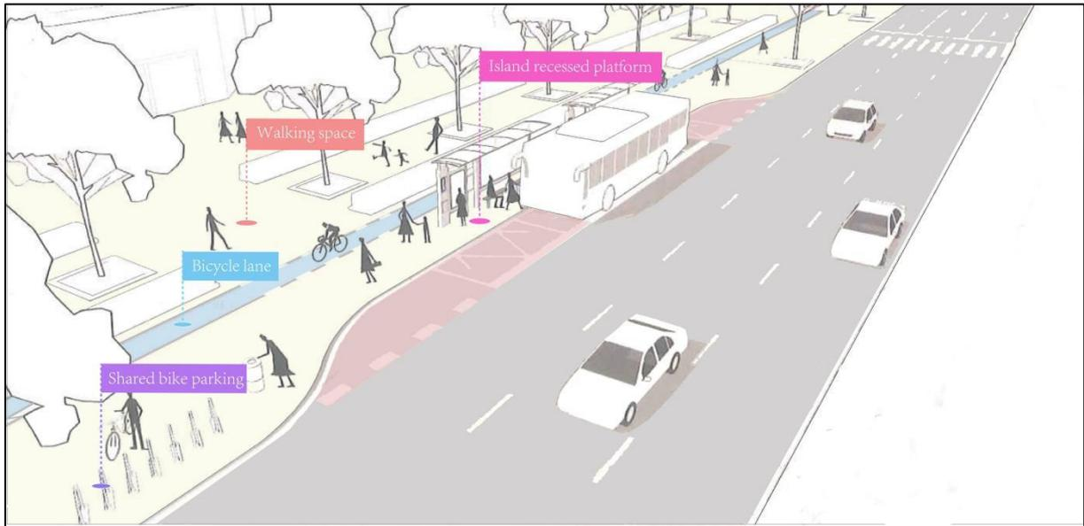
Figure 6-31 Design of bus stop interchange system on city roads around the Racecourse plot
