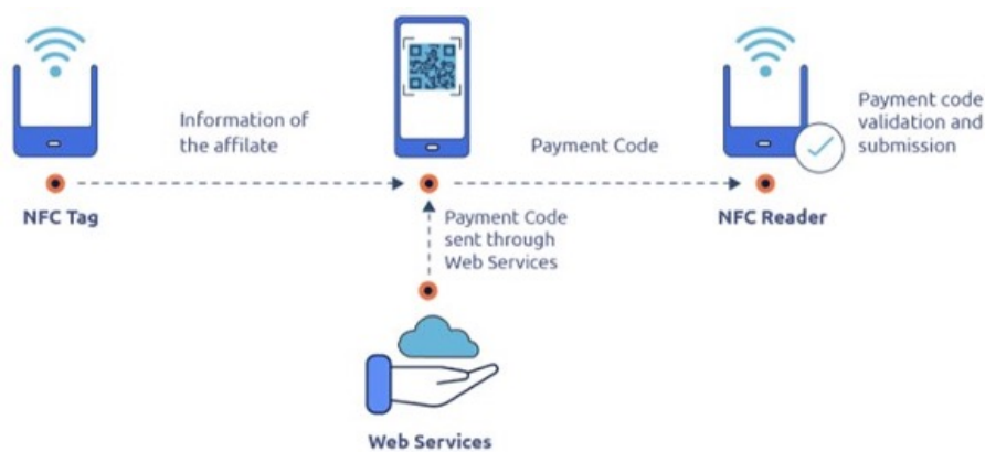
Figure 2.23. Illustrative example of NFC payments functioning. Source: Statista Report 115749 "The many faces of global mobile payments" (2022).
