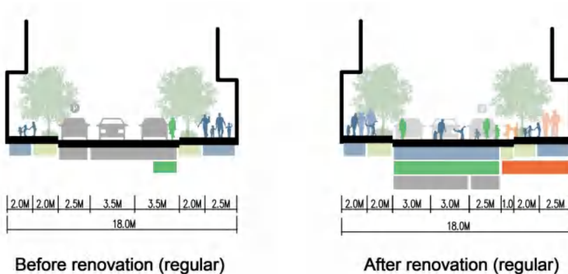
Fig. 7-53 Section of Tiyu West Heng Road before and after renovation II (Drawn by author)
