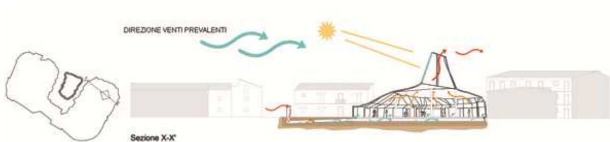
Section functional solar chimney
