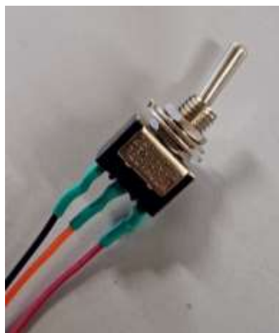
Figure 86. Implied 3-Position Switch Device.
