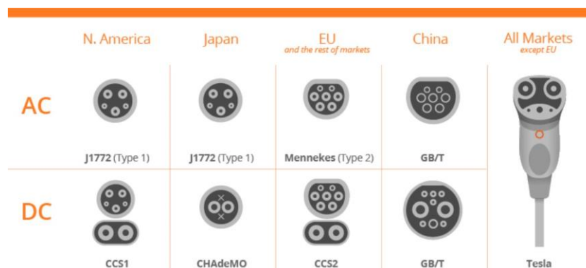
Figura 1: Tipologie di connettori di ricarica ( https://www.connectortips.com/whats-the-status-of-ev-charging-connector-standards )
