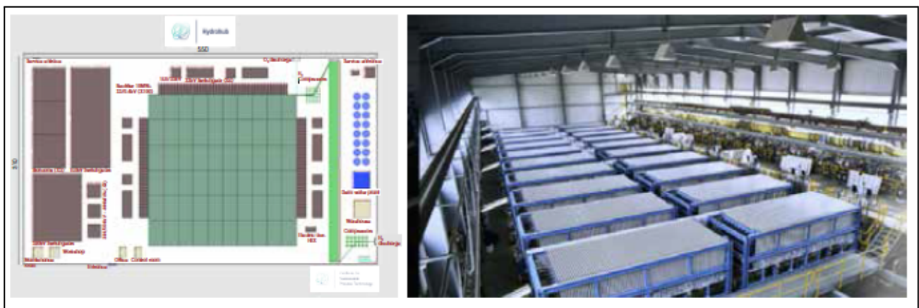
Figure 38 Plot size for an Alkaline 1 GW electrolyzer plant (left) and for a 100 MW Alkaline electrolyser (right) [15]
