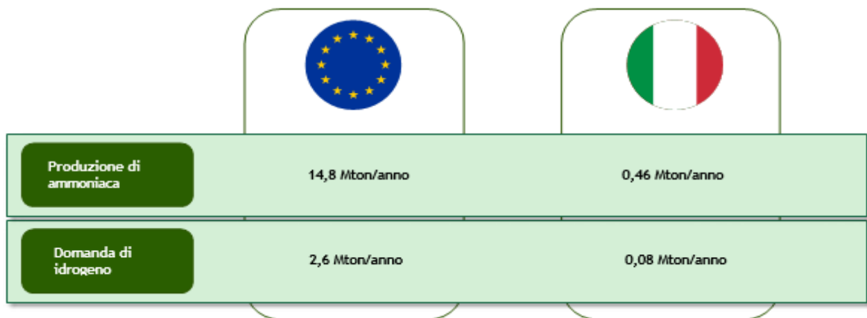
Figure 12 Production and hydrogen demand for ammonia production [12]
