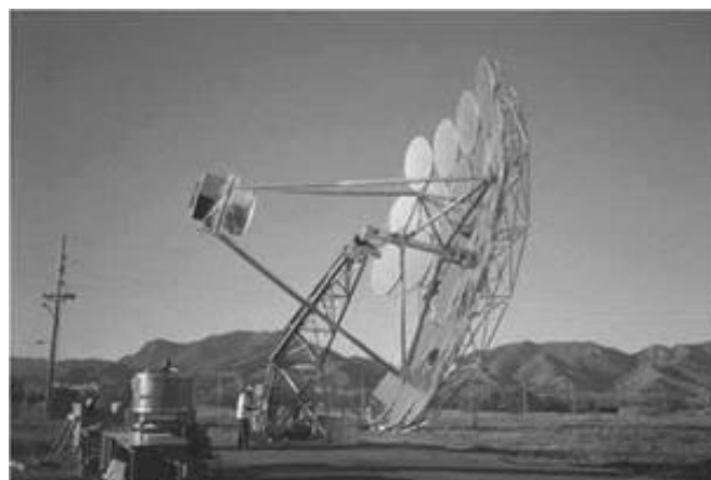
Figura 3.20 – Cummins Power Generation CPG-460 da 25 kW
