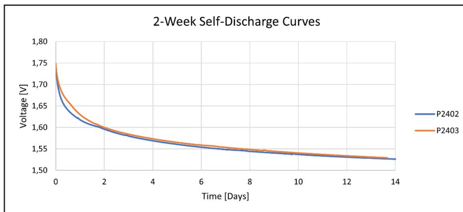
Figure 28 – 2-week self-discharge curves obtained from the non-faulty cycler.
