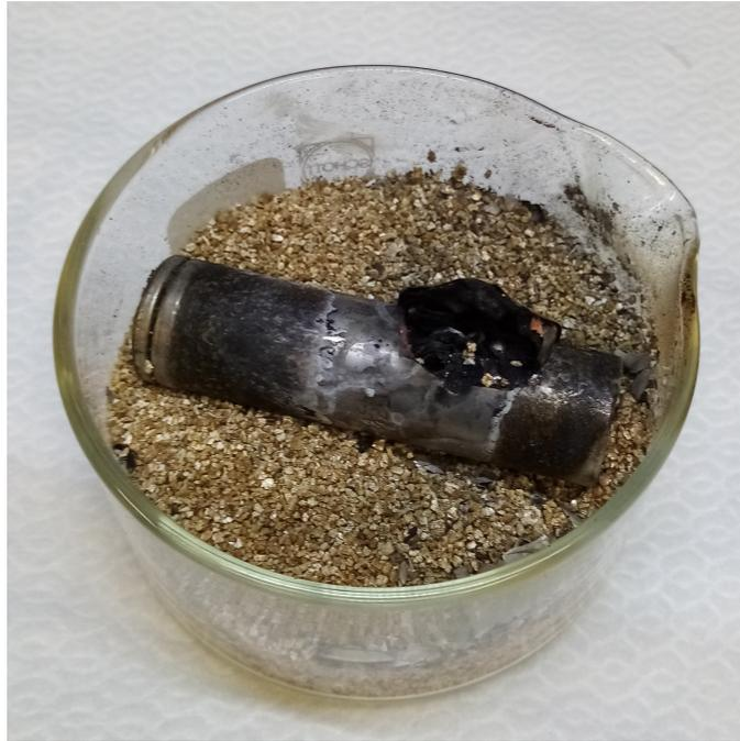
Figure 5.5. Photo of the battery 29E after nail penetration test was performed
