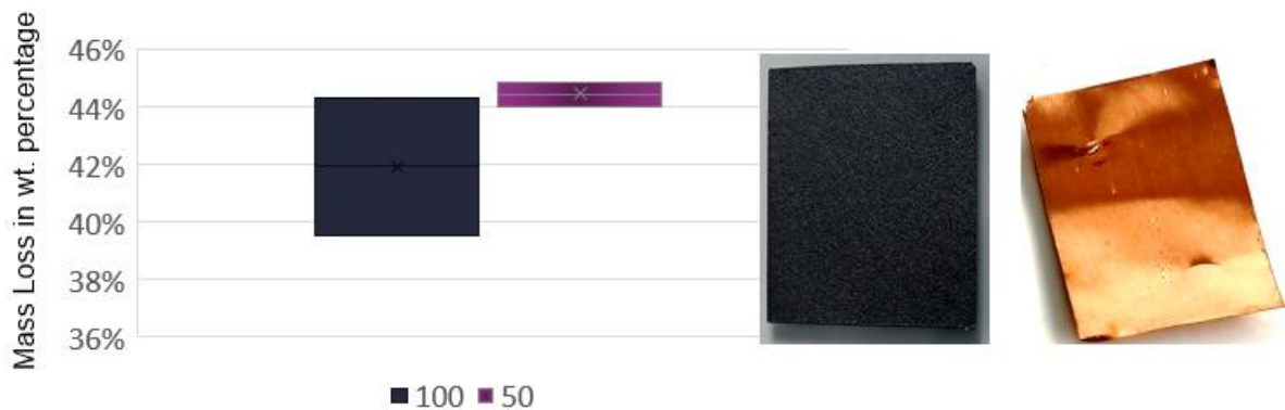
Figure 23 Effect of Power on anode at 37kHz and the optimal removal rate observed at a lower frequency
