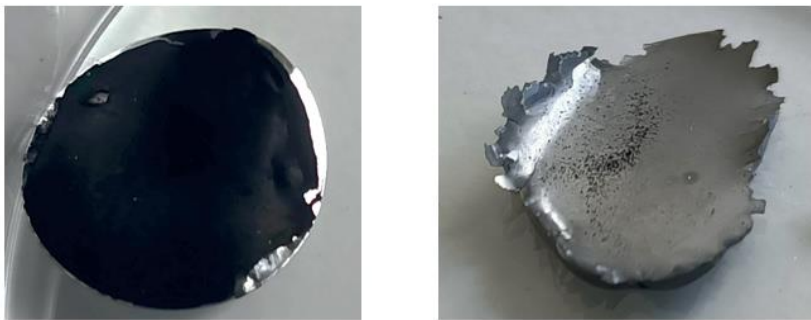
Figure 21 Effect of Power on Cathode at 37kHz and the damaged effect of higher power at a lower frequency
