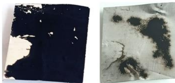
Figure 26 Presence of active material visually observed at ambient temperature
