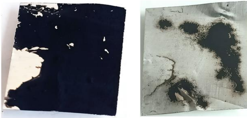
Figure 22 Effect of Power on Cathode at 80kHz and minimised material loss at higher frequency even at a higher power .
