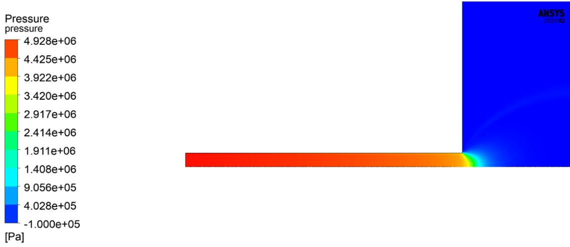
Figure 82: Absolute pressure contour plot of the case with an inlet pressure of 49,28 bar.
