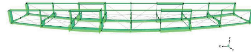
Fig.172:Diagramma Shear 2-2
