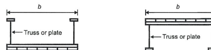
Figure 8.1 – Cross-sections of normal construction decks
