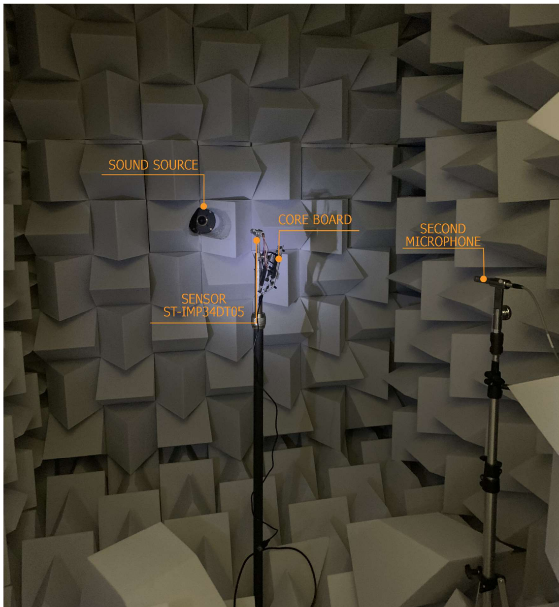
Figure 120 SLP sensor inside the anechoic chamber
