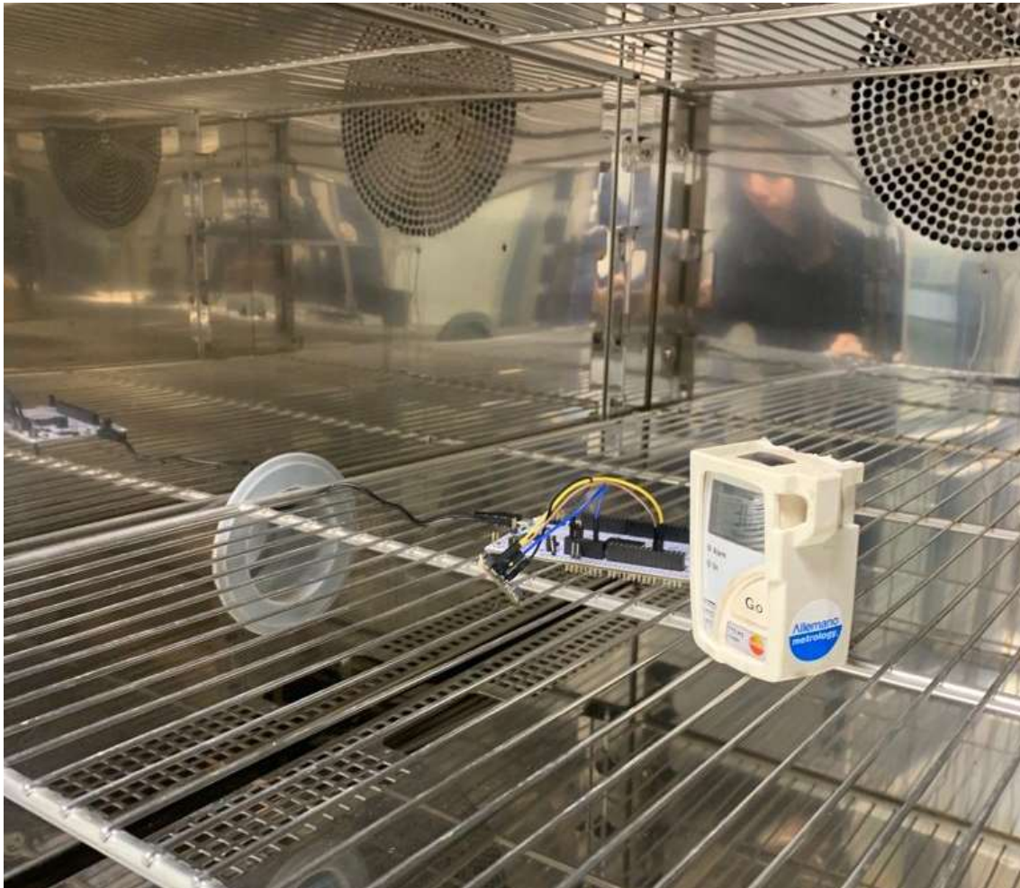
Figure 81 Disposition inside the climatic chamber of the sensor and TESTO 175
