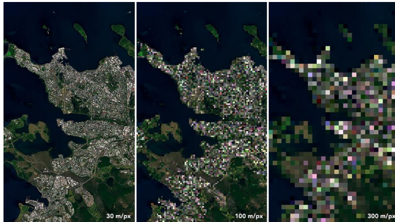
Fig.5-5.Landsat 8 image of Reykjavik, Iceland, acquired July 7, 2019, illustrating the difference in pixel resolution. Credit: NASA Earth Observatory_Source: (EarthData Website of NASA)
