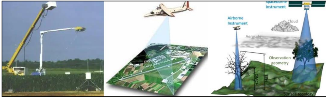
Fig.5-1.(From Left to Right) Ground-Based Platform, Airborne Platform,Space-Based Platform_Source: (The Constructor Website)
