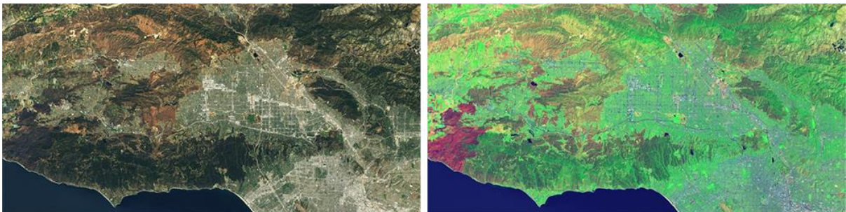
Fig.5-9. Fire scars reflect strongly in Landsat’s Band 7, which acquires data in the shortwave infrared range. The fire scar is not visible in the left image, which is a standard true-colour image. The fire scar stands out clearly in red in the right image, which is a false-colour infrared image. Credit: NASA_ Source: (EarthData Website of NASA)
