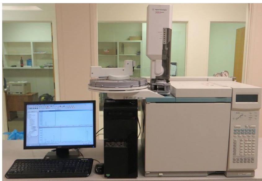
Figura 4.7 Hewlett Packard 6890 FID TCD System
