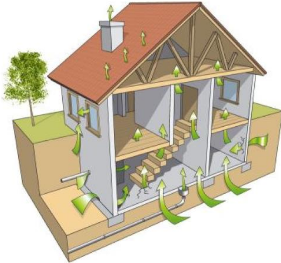
Figure1.17: The incoming Radon from soil [21]
