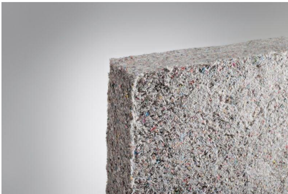
Fig 3.12 Thickness of cellulose insulation
