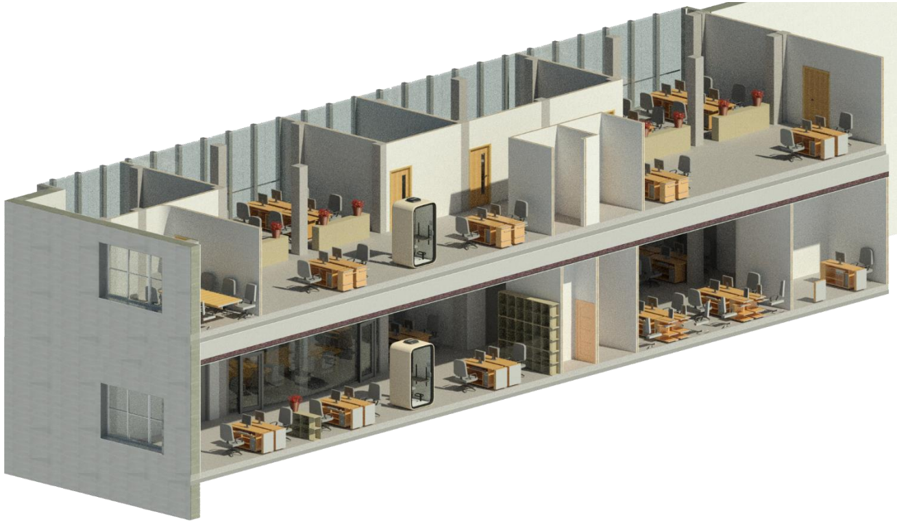
Fig 3.9 3D section of project situation after renovation
