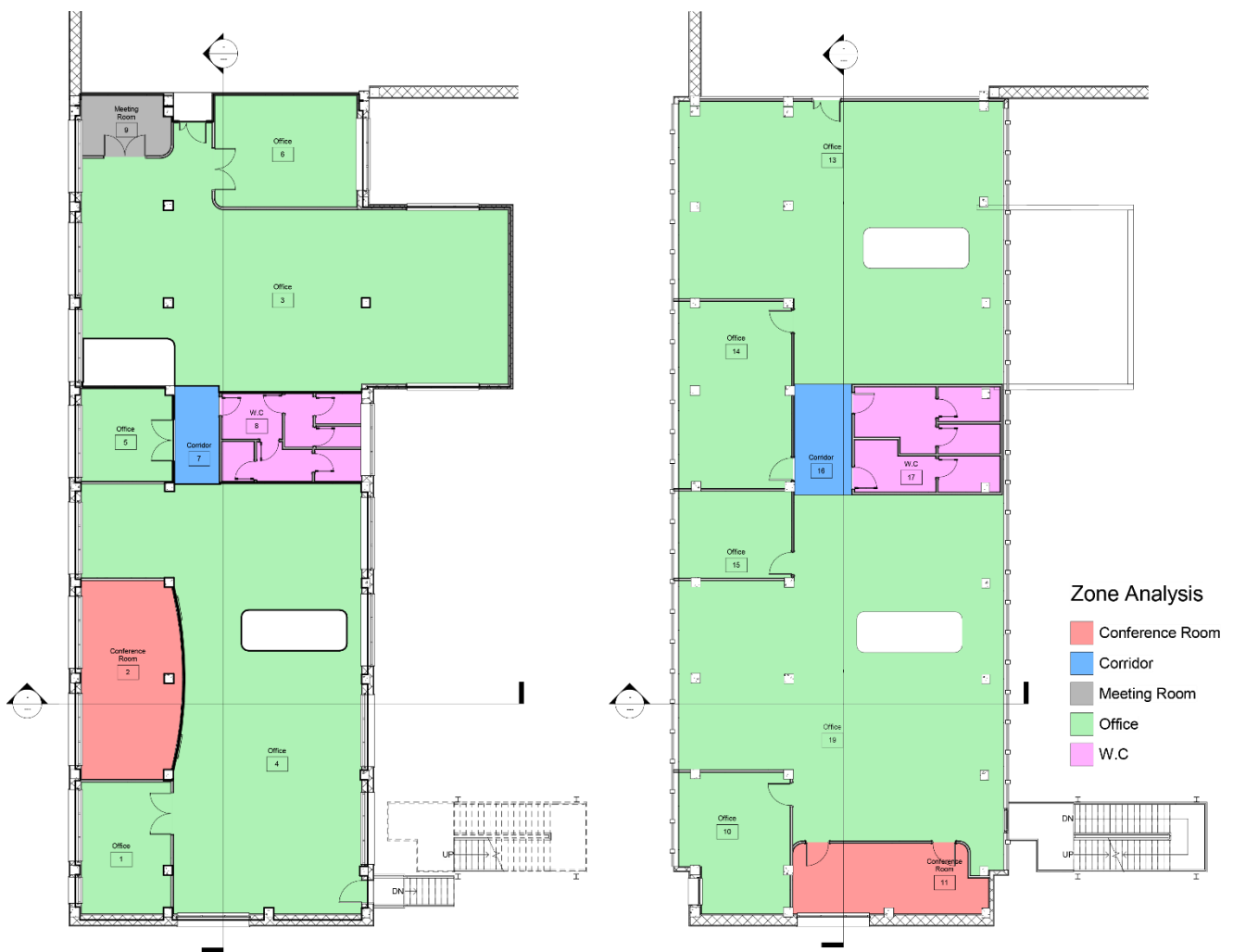
Fig 3.27 Zone of the offices - Project plans
