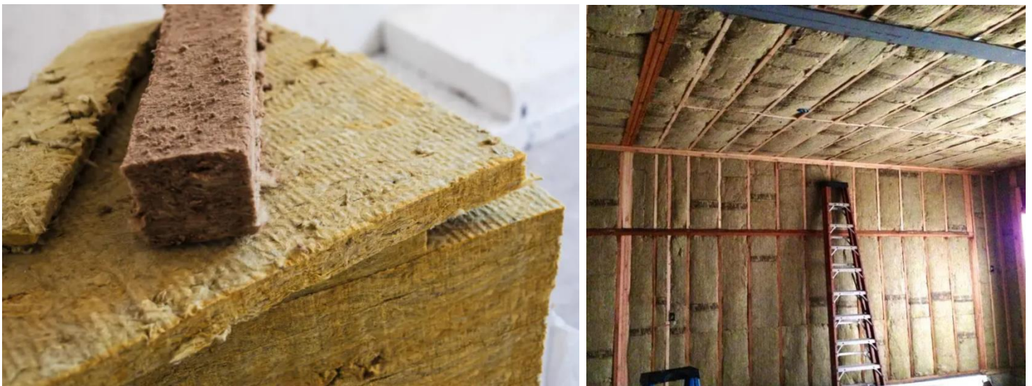
Fig 3.13 Rock wool insulation
