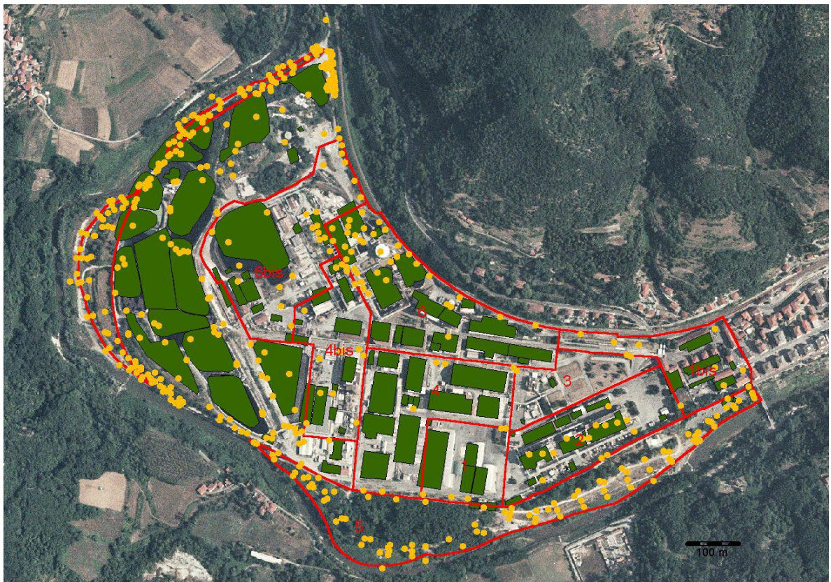
Figure 31. Wells and piezometers
