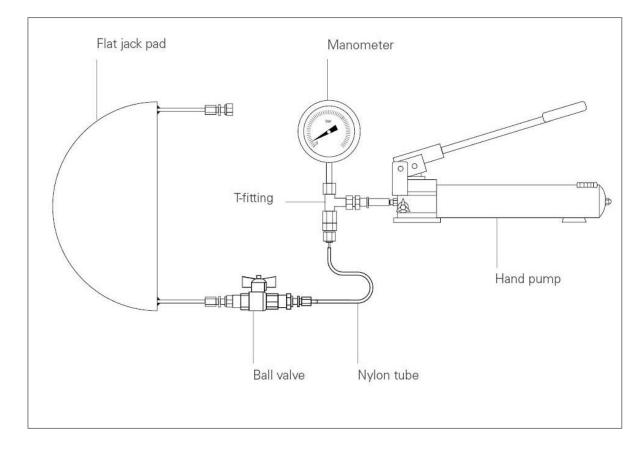
Figure 2.12 Flat-Jack device (www.sisgeo.it)
