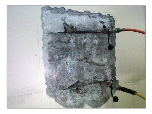
Figure 2.11 Flat-jack test (www.sisgeo.it)
