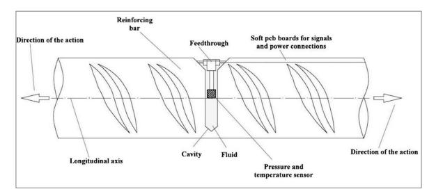
Figure 1.7 smart steel system (Tondolo et al., 2018)
