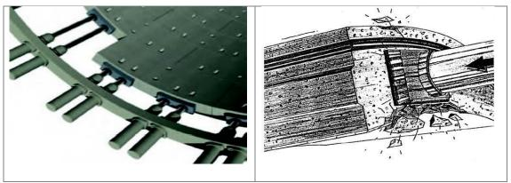
Figure 2.6 Trust jacks pushing on segmental linings (ITA Working Group 2 -Research, 2019)
