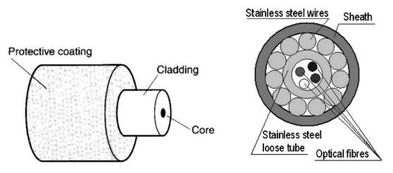
Figure 1.6 Fiber optic wire (Das & Saha, 2018)
