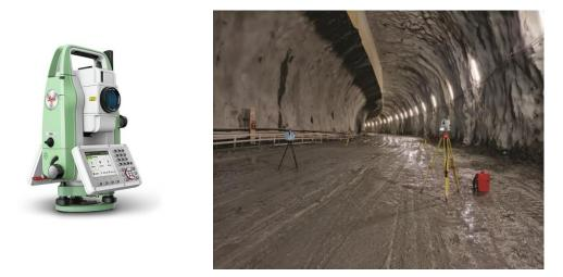
Figure 2.4 Optical monitoring operation with total station (Bilotta et al., 2022)
