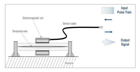
Figure 1.5 vibrating wire strain gauge (ni.com)
