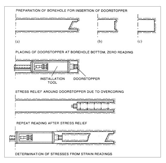
Figure 2.7 Doorstopper test procedure (Ljunggren et al., 2003)
