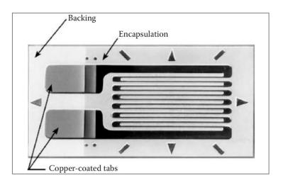
Figure 1.4 Resistive strain gauge (Huston, 2010)
