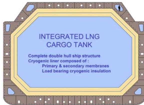
Figure 2.21: Schematic of a membrane tank. Figure taken from [10] with modifications.
