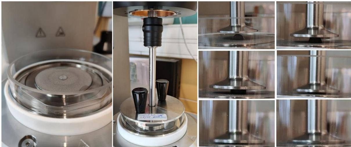
Figure 23 Photos of the analysis procedure. From left to right: Sample placement on the lower plate and loading of deionized water into the channel. Clamping of the moisture-controlled ambient through half covers and upper dish. Flashing of the upper dish to the analysis.
