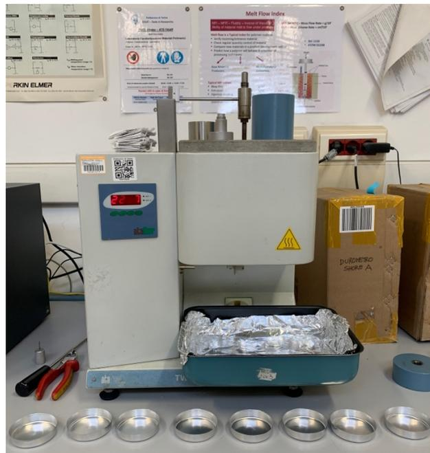
*Figura 2.18 - Plastometro Twelv Index, Ats Faar*
