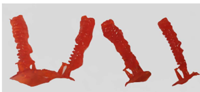
Figure 18 - Not polymerised fusilli using 3DP-F1
