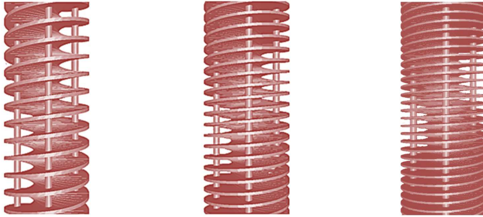
Figure 15 - Fusilli's structure with helix pitch of 4, 2.5 and 1.8 mm, called R1, R2 and R3 respectively.
