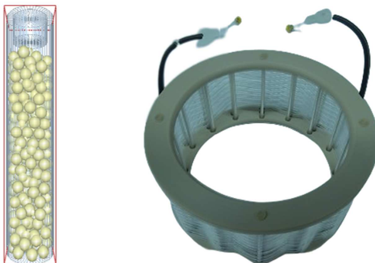
Figure 36 - (Left) Drawn example of PBR; (Right) Coiled tubular reactor of 5 mL volume
