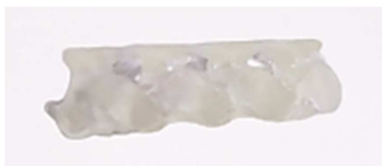
Figure 19 - 3D printed Gyroid with 60% w/w GMA, 40% w/w PETA and 2% w/w BAPO, regarding both GMA and PETA
