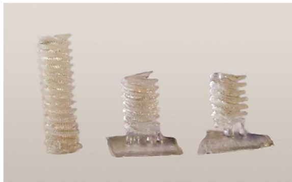
Figure 16 - Formulation development increasing BAPO quantity: (left) 0.5% wt., (centre) 1% wt., (right) 1.5% wt.
