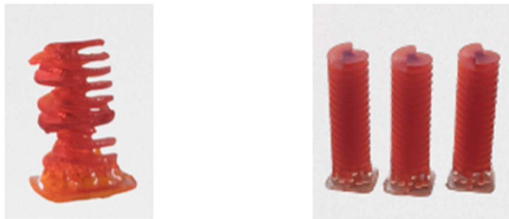
Figure 22 - Fusilli printed vertically with '3DP-F2': (left) lack of polymerization; (right) optimized parameters
