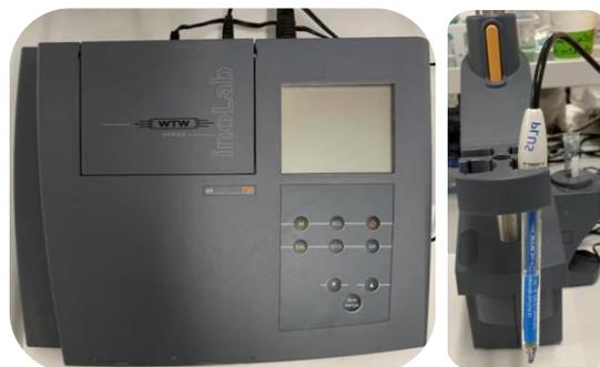
**Fig. 28** Left: pH-meter wtw Inolab 730; Right: electrode Sentix 81.
