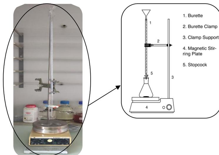
**Fig. 31** Setup used for acid-base titration: burette with magnetic stirrer Heidolph MR 2002 underneath.
