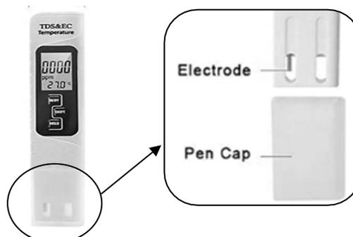
Fig. 29 Conductivity meter TDS&EC.
