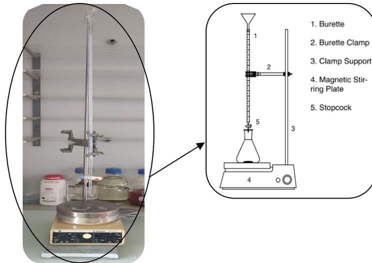
**Fig. 24** Setup used for acid-base titration: burette with magnetic stirrer Heidolph MR 2002 underneath.
