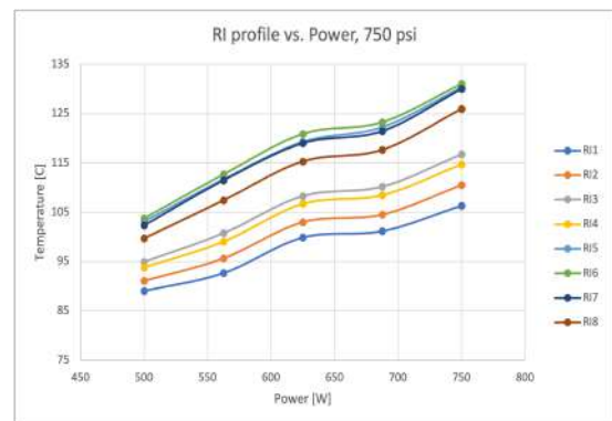
Figure 4.21: RI profiles vs. Power, 750 psi
