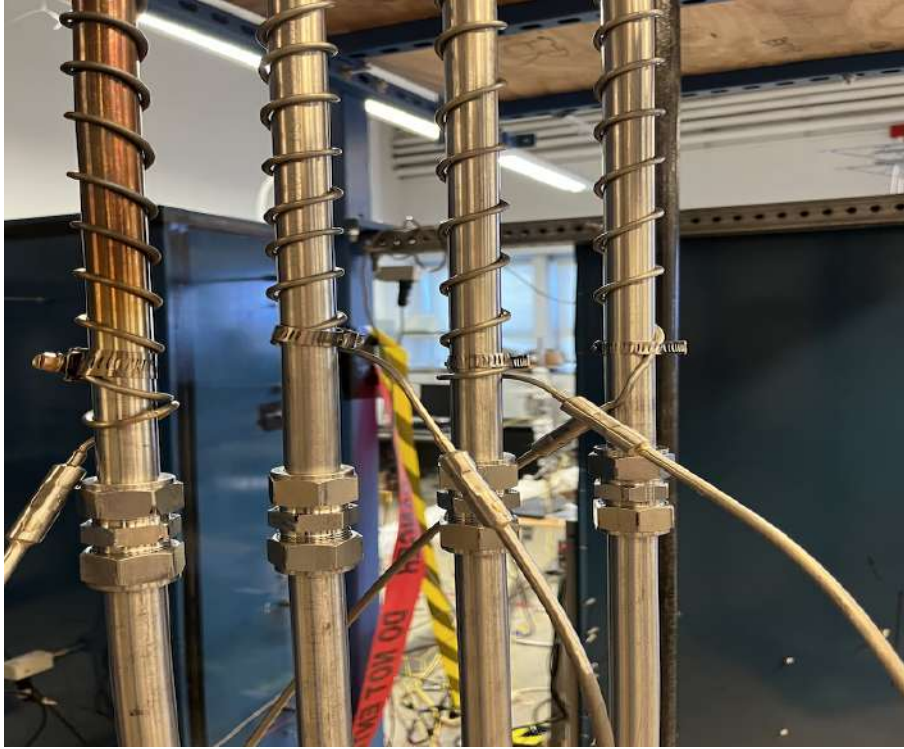
Figure 2.5: Heating coil on riser tubes
