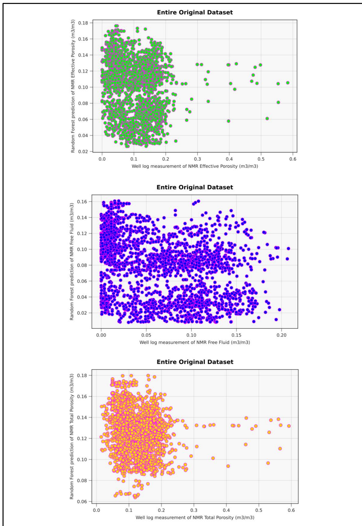
Fig. 3.28: Scatter plots of predicted versus measured NMR porosity, for the RF Model, applied to the Entire Original Dataset of well 1-BRSA-1116-RJS. Plot 1: NMR Effective Porosity (m 3 /m 3 ). Plot 2: NMR Free Fluid (m 3 /m 3 ). Plot 3: NMR Total Porosity (m 3 /m 3 ).
