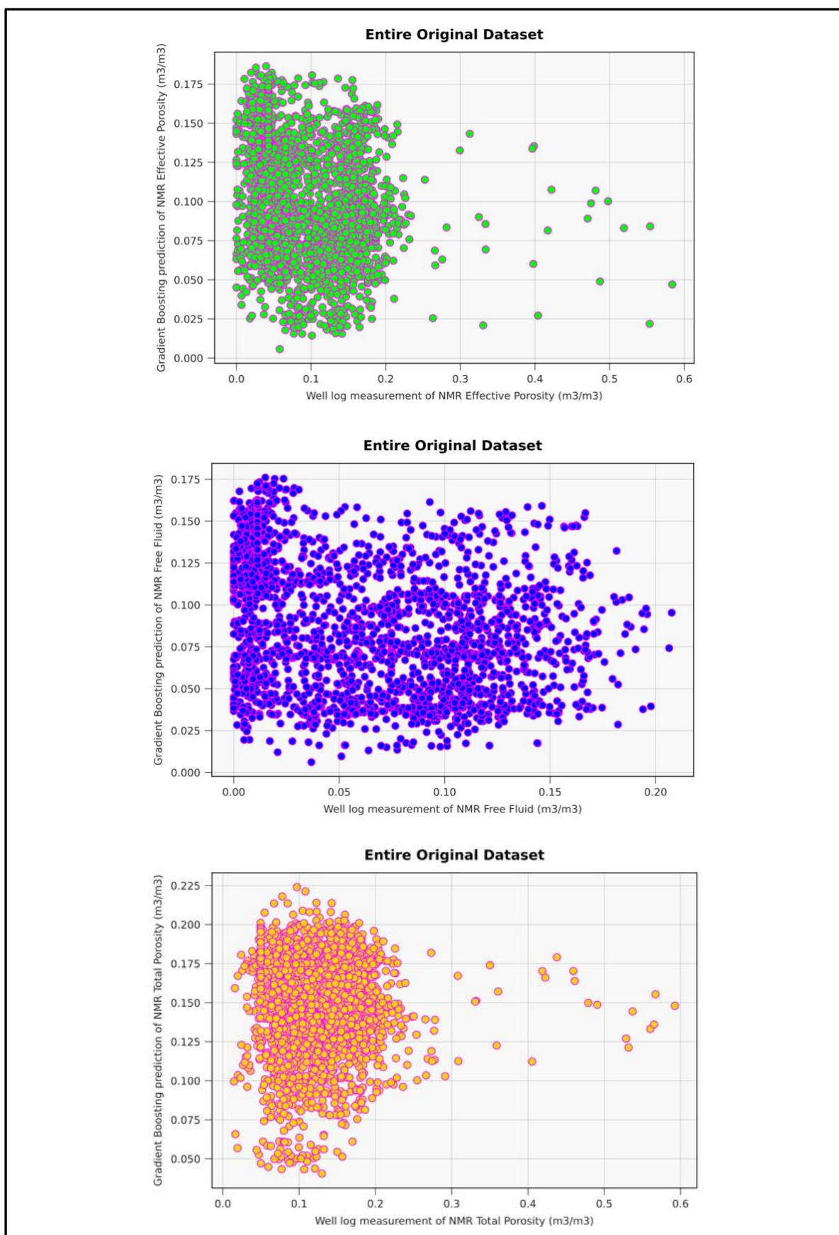
Fig. 3.30: Scatter plots of predicted versus measured NMR porosity, for the GB Model, applied to the Entire Original Dataset of well 1-BRSA-1116-RJS. Plot 1: NMR Effective Porosity (m 3 /m 3 ). Plot 2: NMR Free Fluid (m 3 /m 3 ). Plot 3: NMR Total Porosity (m 3 /m 3 ).
