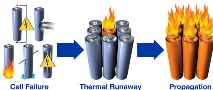
Figure 14 How TR in one cell can lead to destruction of the entire battery [16]
